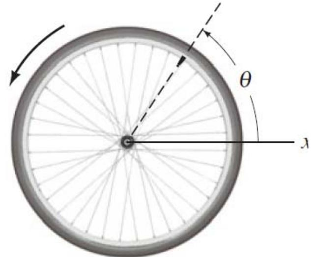
For a rotating disk, the instantaneous linear velocity of a part of the disk far from the axis of rotation is greater than a part of the disk near the axis of rotation. The angular velocity of the two parts are equal (they sweep the same angle over the same amount of time).
