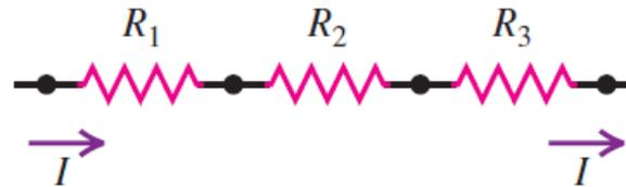
If the resistors are in series, then the current  $I$  must be the same in all of them. The potential difference across the entire combination of the resistors in series is the sum of the individual potential differences across each resistor,
