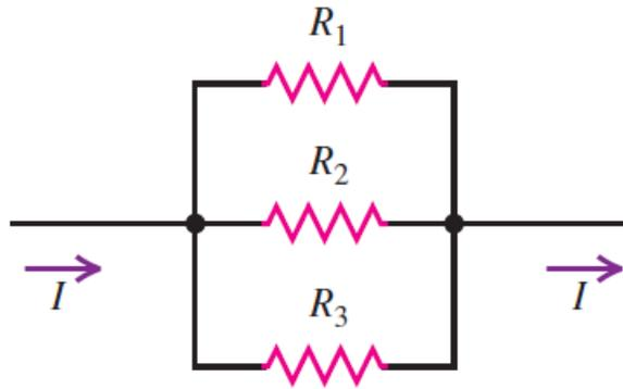
If the resistors are in parallel, then the potential difference between the terminals of each resistor must be the same,
