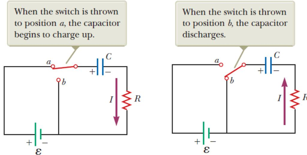
Consider a capacitor of capacitance  $C$  that is being discharged through a resistor of resistance  $R$  as shown in the figure. After how many time constants is the charge on the capacitor one-fourth its initial value?
