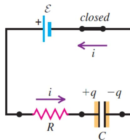
When the switch is closed, the charge on the capacitor increases over time while the current decreases.
