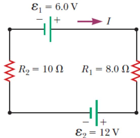
We cannot simplify the circuit by the rules associated with combining resistances in series and in parallel. (If the 10.0 V battery were removed and replaced by a wire from b to the 6.0-V resistor, we could reduce the remaining circuit.) Because the circuit is not a simple series and parallel combination of resistances, this problem is one in which we must use Kirchhoff's rules.
