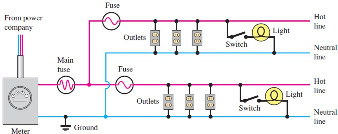
The power company provides three conductors. One is neutral; the other two are both at  $V_{\text{rms}} = 120 \text{ V}$  with respect to the neutral but with opposite polarity ( $180^\circ$  out of phase), giving a voltage between them of  $V_{\text{rms}} = 240 \text{ V}$ .
