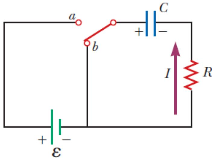
A  $5.00\ \mu\text{F}$  capacitor is charged to a potential difference of  $800\ \text{V}$  and then discharged through a resistor. How much energy is delivered to the resistor in the time interval required to fully discharge the capacitor?
