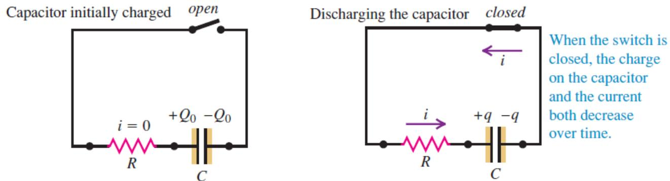
For an initially charged capacitor with initial charge  $Q_0$ , the instantaneous potential differences across the resistor and capacitor given in terms of the instantaneous current  $i$  and charge  $q$  after the switch is closed are
