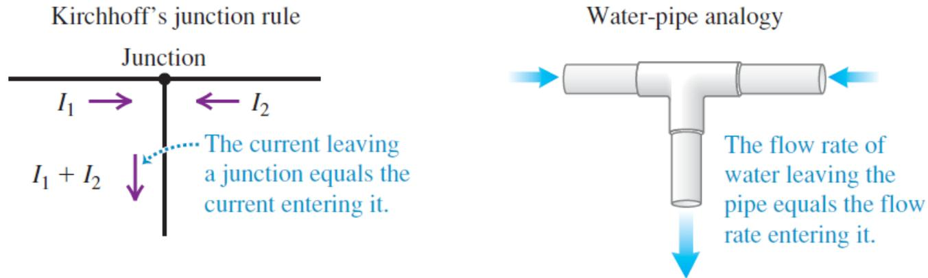
The junction rule is based on conservation of electric charge. No charge can accumulate at a junction.
