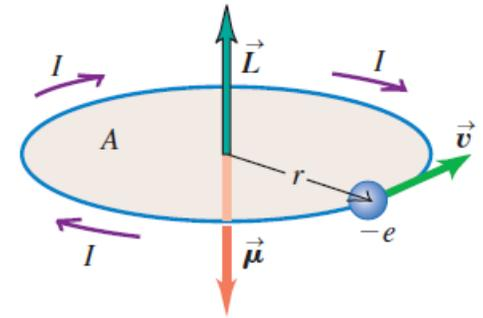
The equivalent current  $I$  is the total charge  $e$  passing any point on the orbit per unit time  $T = 2\pi r/v$ ,
