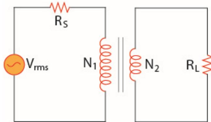
In the ideal transformer circuit shown, the load resistance is  $R_L = 50.0 \, \Omega$ . The turns ratio is  $N_1/N_2 = 2.50$ , and the rms source voltage is  $V_{\text{rms}} = 80.0 \, \text{V}$ . If a voltmeter across the load resistance measures an rms voltage of  $25.0 \, \text{V}$ , then what is the source resistance,  $R_S$ ? <sub>1</sub><sup>2</sup>
