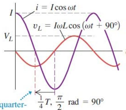
Voltage curve *leads* current curve by a quarter-cycle (corresponding to  $\phi = \pi/2 \text{ rad} = 90^\circ$ ).
