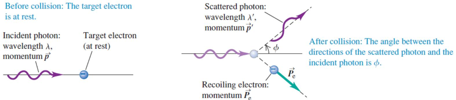
The Compton scattering experiment showed results in which the wavelength change  $\lambda' - \lambda$  is a function of the deflection angle  $\phi$ .
