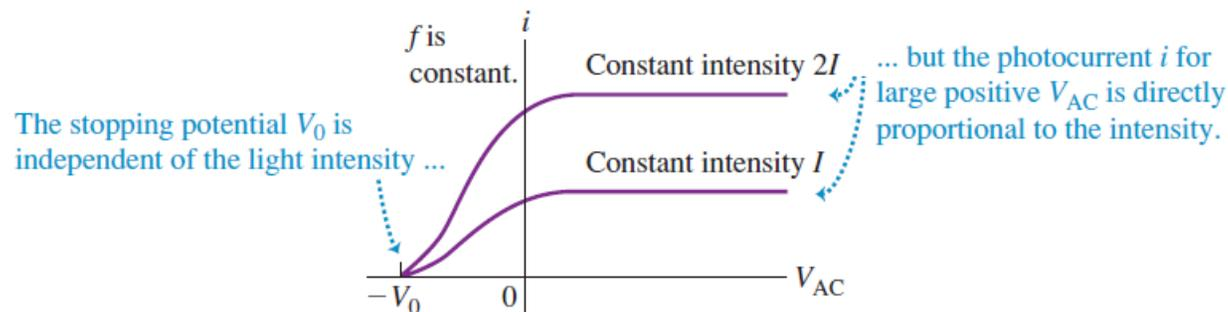
Monochromatic light strikes a metal surface and electrons are ejected from the metal. If the intensity of the light is increased, what will happen to the ejection rate and maximum energy of the electrons?
