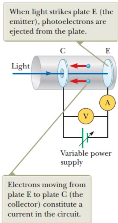
When  $\Delta V$  is equal to or more negative than  $2\Delta V_s$ , where  $\Delta V_s$  is the stopping potential, no photoelectrons reach C and the current is zero.
