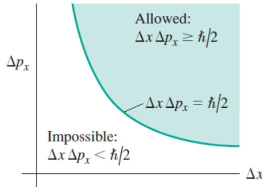
The equation can also be rewritten for energy and time,  $\Delta E \Delta t \geq \frac{\hbar}{2}$ .
