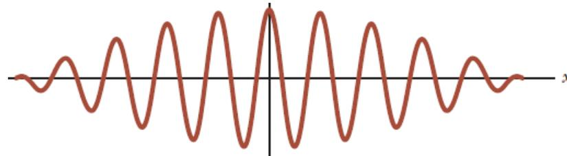
Note that the amplitude is damped on both sides. This damping causes the frequency to be slightly different along the x-direction. Because the momentum is related to the frequency of the photon,  $p = hf/c$ , the momentum is also different along the x-direction. Thus there is some uncertainty in both the position and momentum of the photon.
