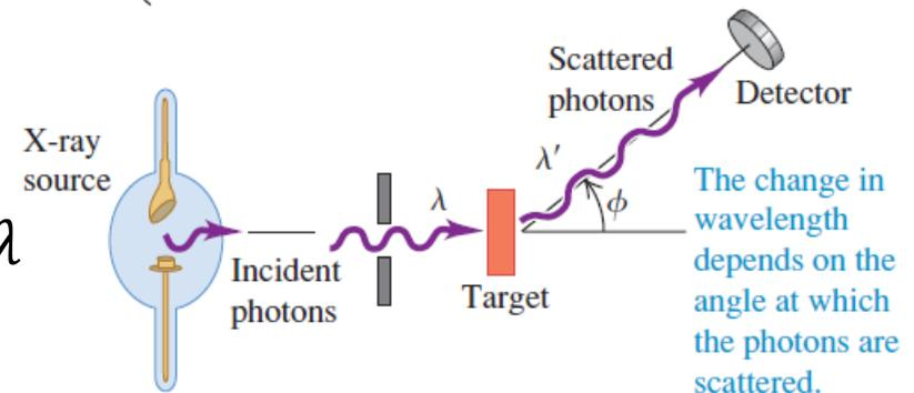
When the photon collides with the electron, it transfers some of its momentum (and energy) to the electron. Thus, the scattered photon should have a lower energy (or lower frequency; longer wavelength). The Compton scattering equation is given by
