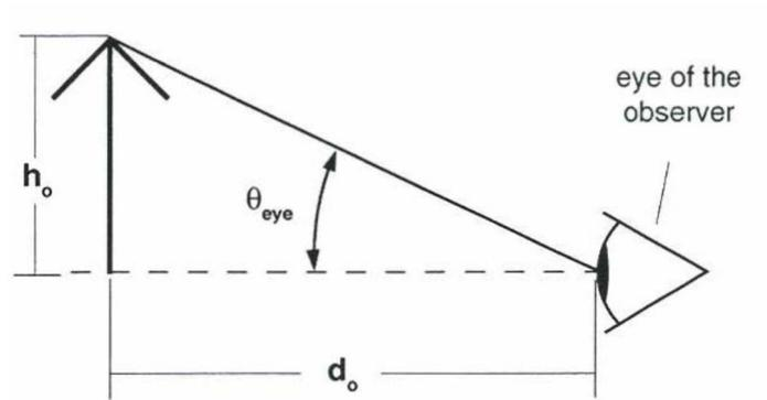
Fig. 2: Diagram for angular magnification.
