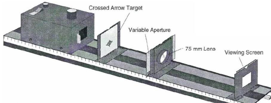
Fig. 3: Diagram for projector experiment.
