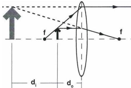
Fig. 1: Ray diagram of lens projection.
