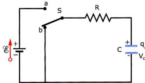
*Fig. 1: Series circuit for charging/discharging a capacitor.*
